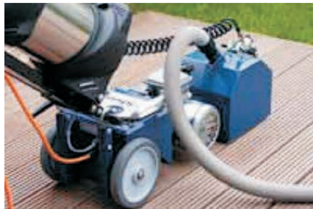
connection of an external dust extractor
