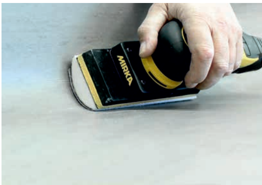
Application in corners and fillets with the round support
